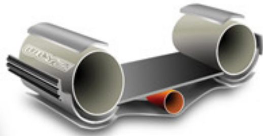
Inflatable V-shaped keel for better navigation and higher stability
