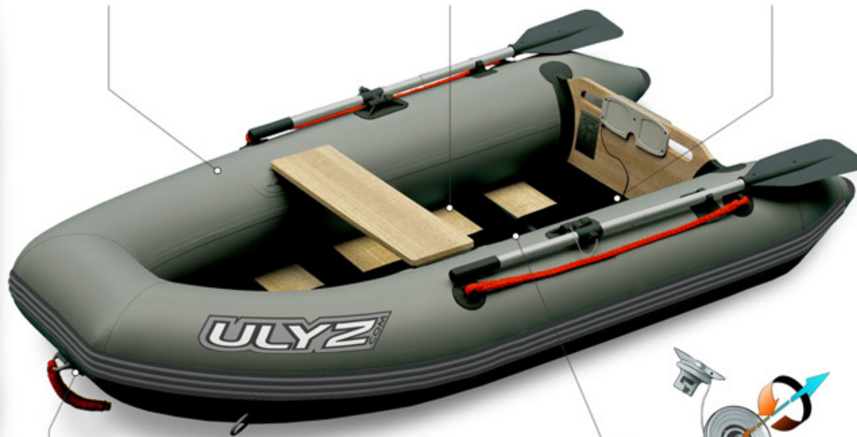
Inflatable V-shaped keel for better navigation and higher stability
